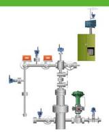
Gas Lift for Oil - controls and optimizes lift gas applied to oil-producing wells to maximize production.
