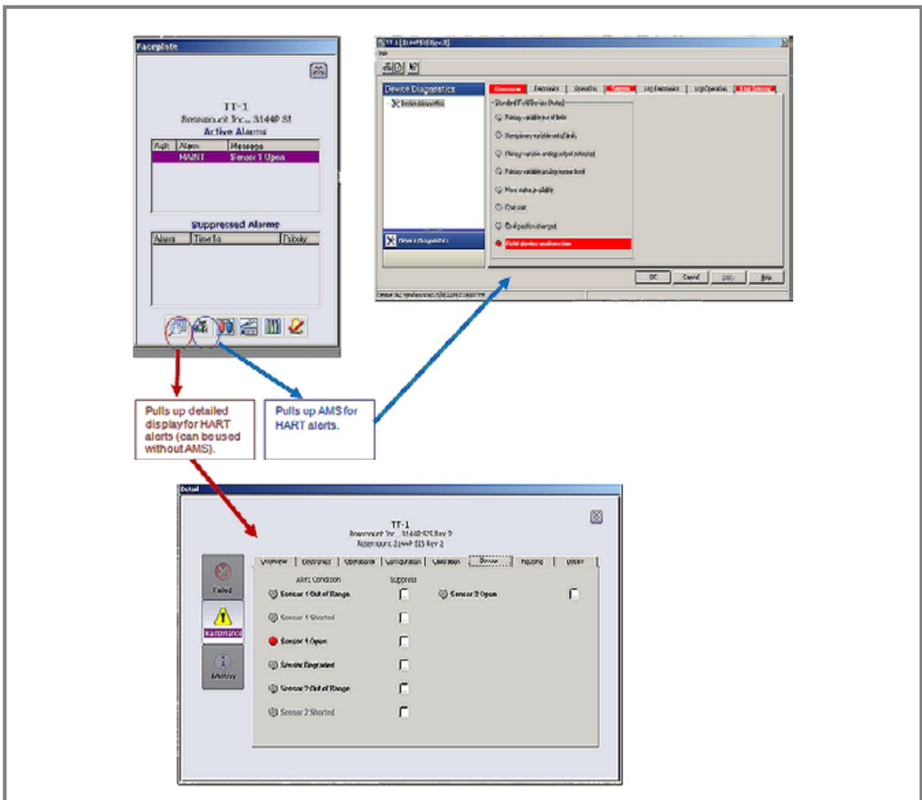
In addition, device alerts are configurable to allow different alarm priorities to exist for different alerts. Configuration is performed by selecting the properties for a HART device from Explorer. From there, the alarms can be enabled and the priorities configured (as shown below).
